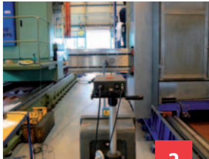
Test of accuracy in positioning (measuring by the laser)
